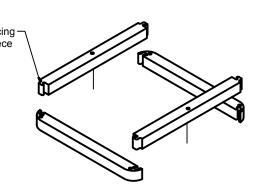
Connect the four pieces using the inward-facing puzzle connectors to form a solid rectangular base.
