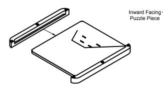
Place the Starlink upside down for outdoor installs or face up for interior mounting. Position each top piece on the sides of the Starlink.
