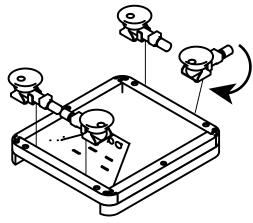
Screw in suction cups or magnets to the inserts on the bottom pieces.
