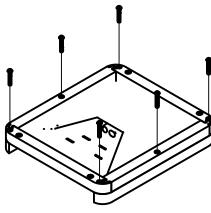
Place the assembled bottom piece on top of the Starlink. Insert M6 bolts through each hole and tighten with the M4 hex key to secure the Starlink.
