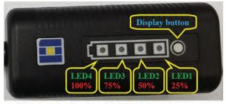
\*When the capacity is lower than 10%, LED1 will flash.
