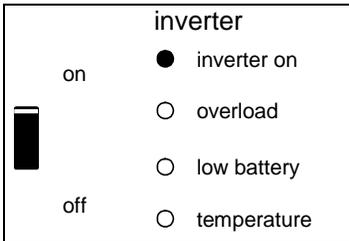
The inverter is on and supplies power to the load.
