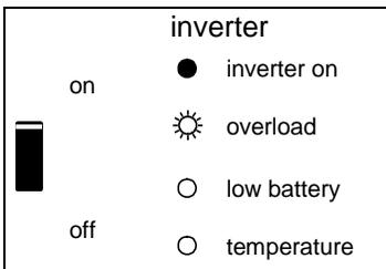
The nominal output of the inverter is exceeded. The "overload" LED flashes.
