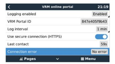
If a Connection error is shown, the VGX is not able to contact the VRM database. The connection error will show an error code that indicates the nature of the connectivity problem. Also, details of the error message are shown, to facilitate on site IT experts to diagnose the problem.
