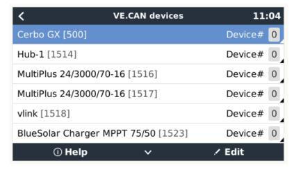
Each entry first shows the name - either the product name as in our database, or when configured, the custom name as configured during installation.
