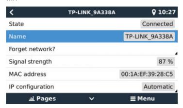
When using Wi-Fi and the menu shows 'No Wi-Fi adapter connected' check the USB connection to the Wi-Fi dongle. Try to remove the dongle and insert it again.
