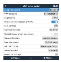
The transmission of the data logs has been designed to work also on bad internet connections. Lines of up to 70% permenant packet loss are still sufficient to get the data out, even if delayed in some cases.
