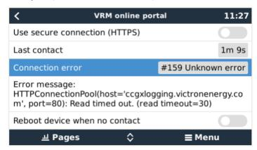
Check 'Last contact'. If this shows dashes, the GX device has not been able to contact the VRM Portal since power up. If it shows a time, but still an error is shown, then the GX device has been able to send data, but has since lost contact.
