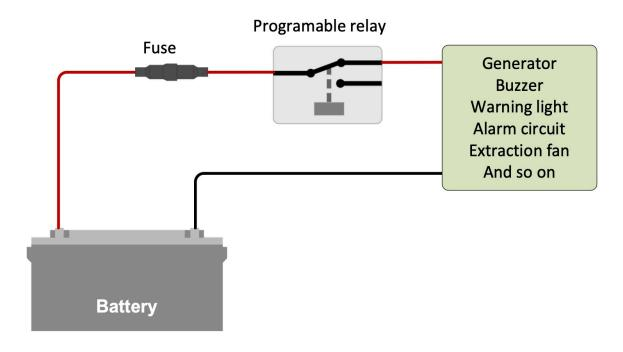
Figure 2. Programmable relay wired to operate as a potential free contact switch
