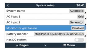
The alarm shows as a Notification in the GUI, and as an alarm on the VRM Portal, and is available on ModbusTCP / MQTT.
