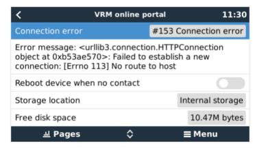
• Error #153 Connection problem, and then specifically an SSL related issue, such as in below screenshot: check the date and time setting of the Gx Device, and also the time zone. And check that your router router is not showing a special disclaimer, login or acceptance page, like often seen in airports, hotels and other public wifi.
