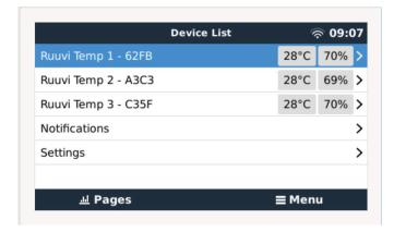
The temperature relay is controlled from Settings Menu -> Relay -> Function (Relay 1/2) -> Temperature
