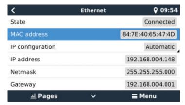
When using Ethernet and State shows 'Unplugged', verify that the Ethernet network cable is not faulty: try another one. The two lights at the back of the VGX, where the Ethernet RJ45 cable plugs in, should be lit or blinking. Two dead lights indicate a connection problem.
