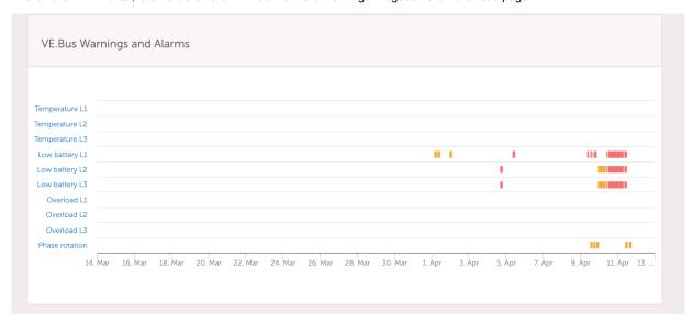
And also it will be listed in the Alarm Log on VRM, and an email will be sent; using the VRM Alarm Monitoring system.
