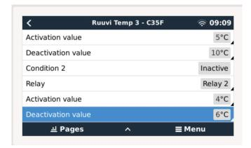
This will mean that Relay 1 will be active if the battery temperature falls to 5 degrees. If the temperature continues to fall below 5 degrees to 4 degrees, then the second heat pad will be engaged via Relay 2.
