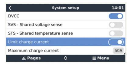
This setting is available in the "Settings → "System Setup" menu on the GX device.
