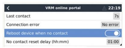
This feature, disabled by default, makes the GX device automatically reboot itself in case it has not been able to connect to the VRM Portal.
