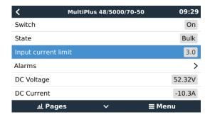
The limit as set by the user in the VGX will be applied to all inputs where 'Overruled by remote', configured with VictronConnect or VEConfigure, is enabled:
