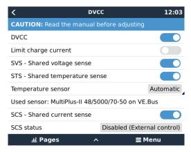
**Example 1 - Managed CAN-bus batteries** For example, in systems with an Managed CAN-bus BMS battery connected, the GX receives a Charge Voltage Limit (CVL), Charge Current Limit (CCL), Discharge Current Limit (DCL) from that battery and relays that to the connected inverter/chargers and solar chargers. These then disable their internal charge algorithms and simply do what they're told by the battery. There is no need to set-up charge voltages or choose the charge algorithm type.
