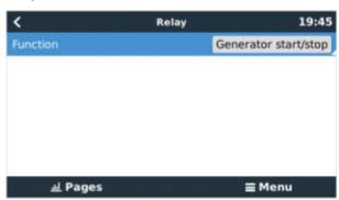
Now that has been enabled, all the settings pertaining to the Automatic Generator Start/Stop function will be found in the main Menu under: Settings  $\rightarrow$  Generator start and stop.
