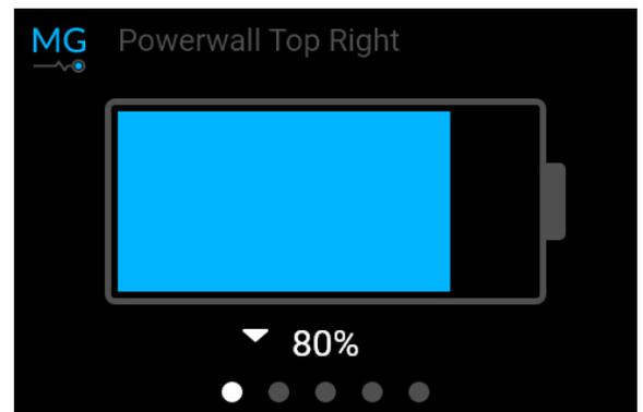
The minimal start page is one of the two options for the default start up screen of the Energy Monitor. From the factory, the monitor will use minimal start as the start screen.
