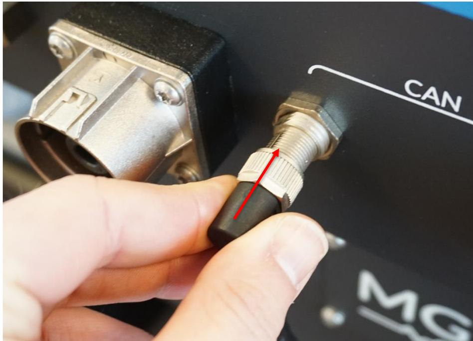
3. Lock the connector by rotating the locking nut clockwise. Hand-tightened will be sufficient, do not use tooling to tighten.
