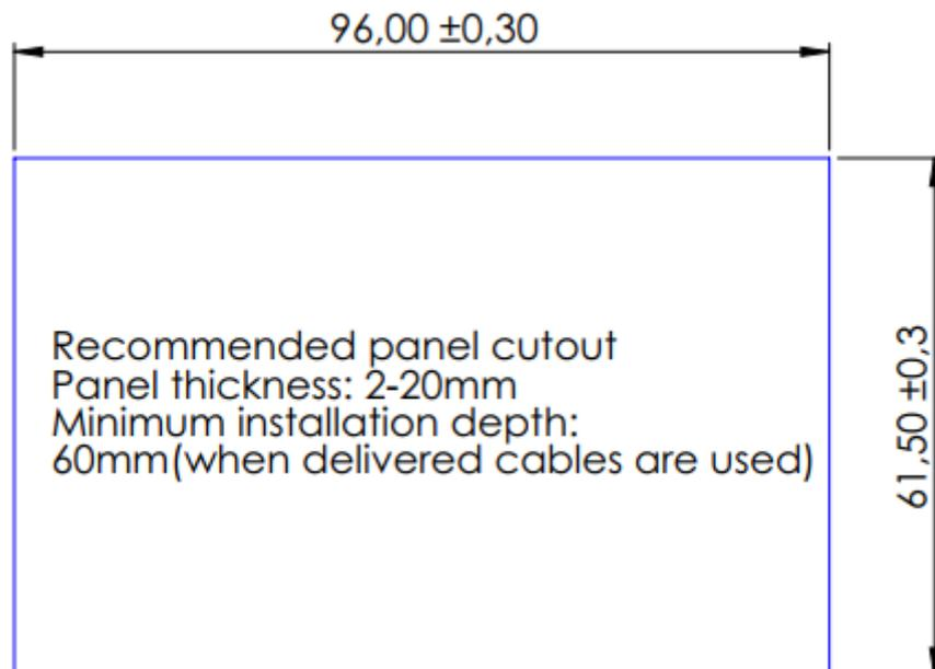
Figure 6 - Panel cut-out in mm
