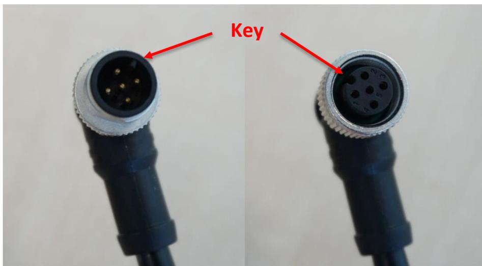
2. Bring the connections face of the cable connector up the device connector in such a way that the position of the key matches to that of the opposing connector.
