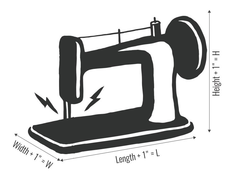
Measure length, width, and height on your machine. Add 1" to each measurement to find your value for L, W, and H.
