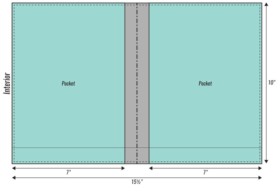
Note: Cover liner is made from 10" squares, 10" x 6½" rectangle and (2) 10½" x 1¾" rectangles to make a 10½" x 16" lining.
