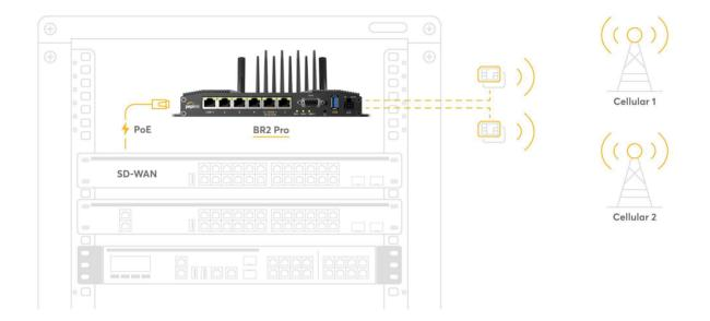
For example, the MAX BR2 Pro can act as a dual LTE/5G connectivity. By powering up the MAX BR2 Pro with a PoE output from your current SD-WAN infrastructure, you can add a dual LTE/5G connectivity to your SD-WAN infrastructure without extra configuration.
