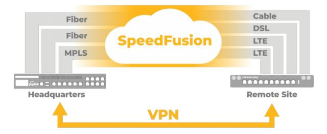
Peplink Balance SpeedFusion<sup>™</sup> Bandwidth Bonding is our patented technology that enables our SD-WAN routers to bond multiple Internet connections to increase site-to-site bandwidth and reliability. SpeedFusion securely connects one or more branch offices to your company's main headquarters or to other branches. The data, voice, and video communications between these locations are kept confidential across the public Internet.
