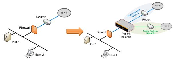
Enable drop-in mode using the Setup Wizard. After enabling this feature and selecting the WAN for drop-in mode, various settings, including the WAN's connection method and IP address, will be automatically updated.
