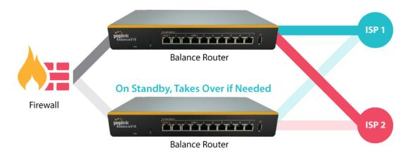
When your organization has a corporate requirement demanding the highest availability with no single point of failure, you can deploy two Peplink routers in <u>High Availability mode</u>. With High Availability mode, the second device will take over when needed.
