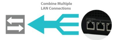
Use 802.3ad to combine multiple LAN connections into a virtual LAN connection. This virtual connection has higher throughput and redundancy in case any single link fails.
