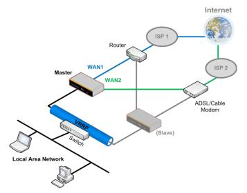
In the diagram, the WAN ports of each Peplink Balance unit connect to the router and to the modem. Both Peplink Balance units connect to the same LAN switch via a LAN port.
