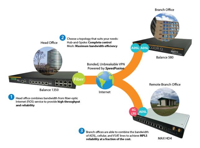
Achieve faster speeds and greater reliability while paying only 20% of MPLS costs by connecting multiple ADSL, 3G, and 4G LTE links. Choose a topology that suits your requirements: a hub-and-spoke topology maximizes control over your network, while a meshed topology can reduce your bandwidth overhead by enabling your devices to form Unbreakable VPN connections directly with each other.
