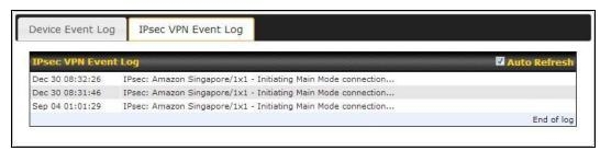
This section displays a list of events that have taken place within an IPsec VPN connection. Check the box next to **Auto Refresh** and the log will be refreshed automatically.
