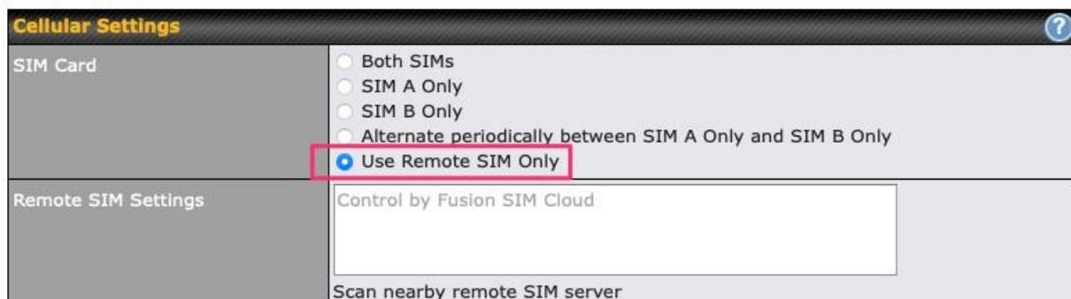
4. Enter configuration settings in the **Remote SIM Settings** section. Click on **Scan nearby remote SIM server** to show the serial number(s) of the connected SIM Injector(s). Available configuration options for cellular interface are shown below:
