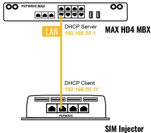
This is the most basic scenario in which the SIM Injector is connected directly to the cellular router's LAN port via an ethernet cable. This allows for the cellular router to be positioned for the best possible signal. Meanwhile, the SIM cards can be conveniently located in other locations such as the office, passenger area, or the bridge of a ship. The SIM Injector allows for easily swapping SIM cards without needing to access a cellular router.
