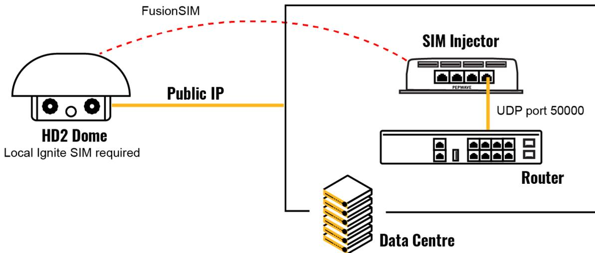
Requirements for installing a SIM Injector in a remote location:
