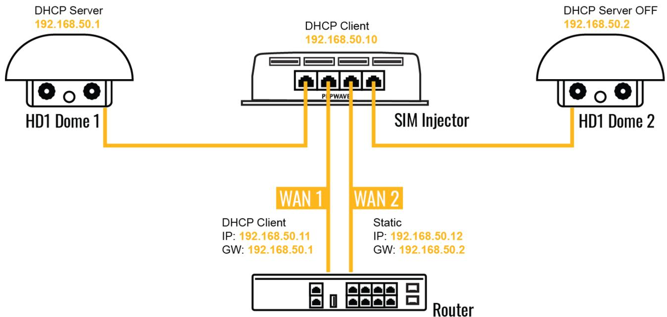
In this scenario, each HD Dome creates a WAN connection to the main router. A single SIM Injector is used to provide SIM cards for each HD Dome. The HD Dome can be replaced with any Peplink cellular router supporting RemoteSIM technology.
