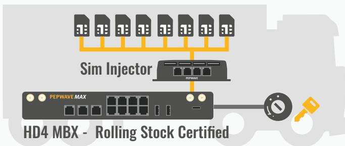
The HD4 MBX comes with multiple features to make it ideal for on-the-go deployments. Ignition Sensing gives it the ability to turn on and off depending on whether the vehicle has started. Upon vehicle shutdown, the MBX can also shut down after a user-defined interval, saving the battery from excessive drain.
