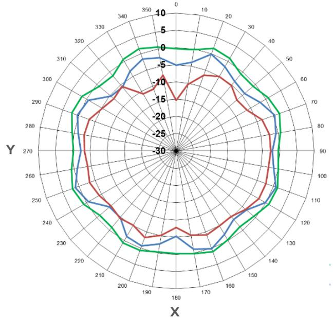
Note: Gain values at 2° elevation indicated are without cable loss. Please refer to the electrical specs chart to include cable losses.
