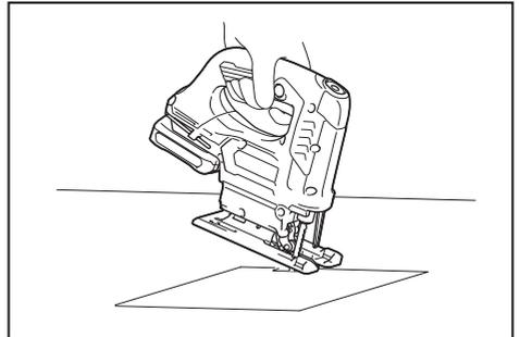
You need not bore a starting hole or make a lead-in cut if you carefully do as follows.
