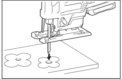
For internal cutouts without a lead-in cut from an edge, pre-drill a starting hole 12 mm (15/32") or more in diameter. Insert the jig saw blade into this hole to start your cut.
