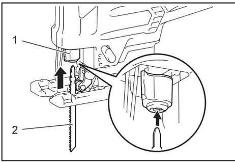
► 1. Jig saw blade holder 2. Jig saw blade
