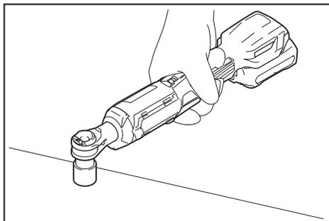
The tool also works without socket. The adaptor hole can fasten M8 (5/16") bolt/nut. (works as 13mm socket)
