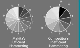
Synchronized RPM and BPM prevents overlapping impacts for up to 50% more efficient drilling
