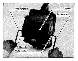
CAUTION: The output shaft has a left hand thread.
