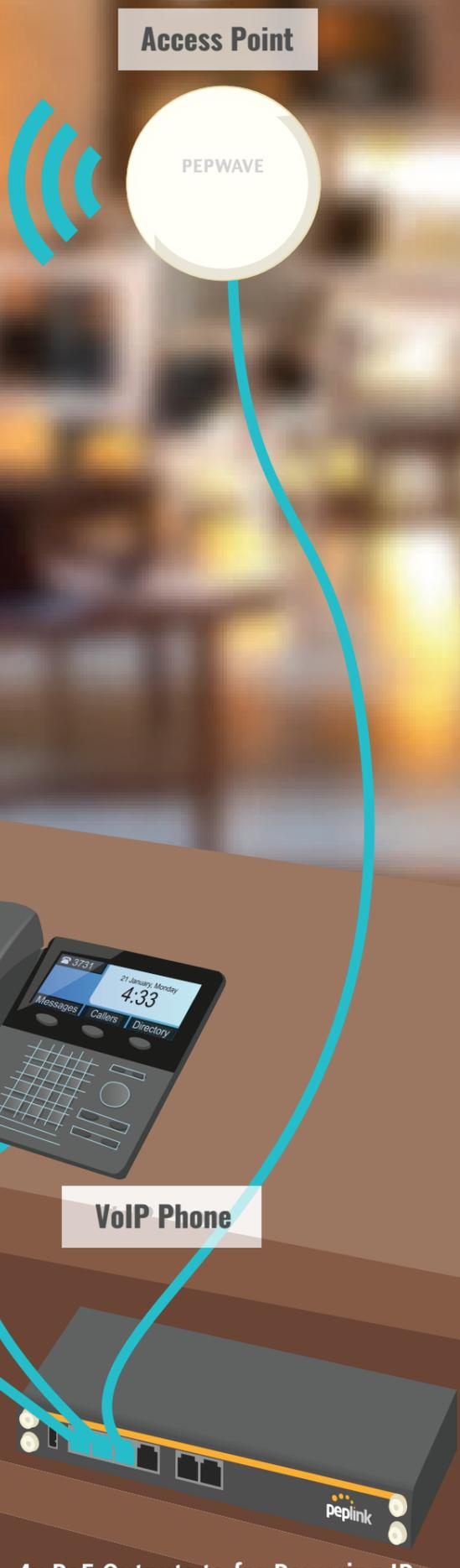
4x PoE Outputs to for Powering IP Phones, PoS Terminals, and Access Points (Requires PoE Activation Kit)
