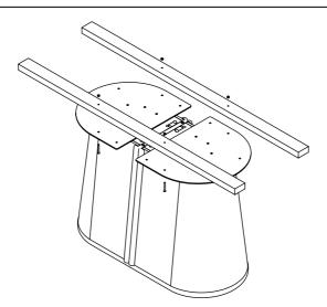
Remove Nuts and Bolts of transport lift rails and remove lift rails. Return to warehouse/dispose of lifting rails and hardware.
