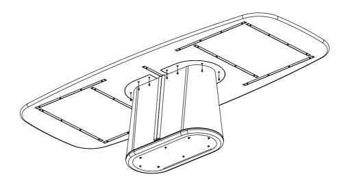
Use supplied Countersunk M6 bolts and secure top to mounting plate. Ensure all bolts are tightened accordingly.
