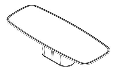
With the appropriate number of people, place top on top of mounting brackets. Ensure to align mounting brackets to brackets pattern in top.
