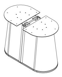
**3** Before placing top on base, check base for any marks and/or damage.
