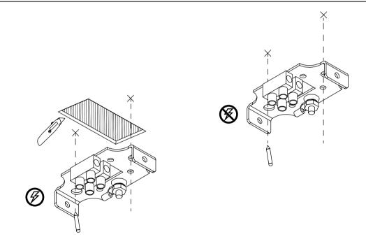
With a pencil, mark fixing holes either side of the central markings. Cut hole in ceiling for driver at one central marking point. Only one ceiling rose required for electrical connection.
