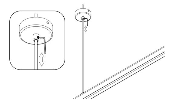
8 Loosen cable grip with allen key. Adjust ceiling cables to desired length and tighten cable grip.
