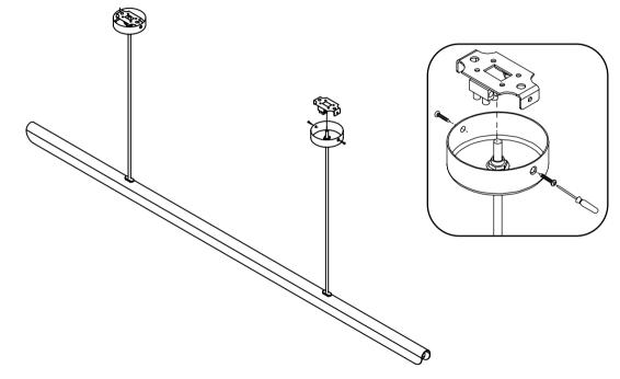
**2** Remove ceiling bracket from ceiling rose by unscrewing screws.
