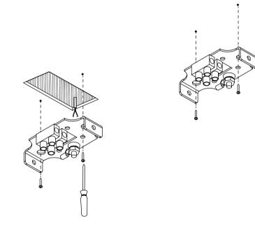
Screw the ceiling bracket onto the ceiling, ensuring there is enough cable exposed from driver to connect both positive and neutral connections into the terminal block. Use the integrated terminal block on the ceiling bracket to connect wiring.
