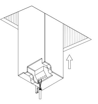
**6** Making electrical connections and secure driver in ceiling cavity.
