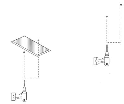
5 Drill holes and use appropriate ceiling fixings.
