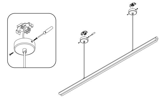
9 Connect cabling to terminal block. Raise ceiling rose to ceiling bracket and use supplied screws to secure.
