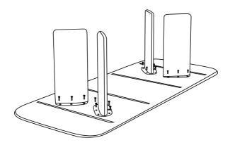
Align leg plates with rebated sections and ensure they are sitting flush. Using provided Hex bolts, screw clockwise into the countersunk holes in the plate. Ensure bolts are firmly tightened.
