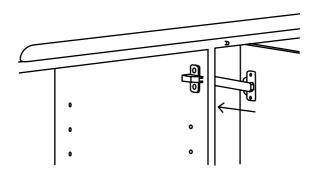
Unwrap shelves and doors (packaged separately) and lay on soft surface. Clip brackets on doors into their respective fittings, ensuring doors are orientated the right way up. These clip onto the face of the internal bracket.
