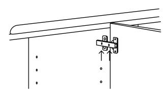
Level doors using the 2 screws to adjust height, angle and protrusion.
