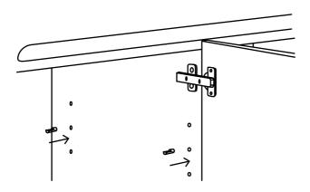
Insert shelf inserts into respective holes inside the cabinet with the flat spots facing up. Height can be set using the suitable holes.
