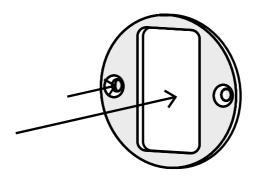
Offer the Wall Bracket up to the wall and fix both points using appropriate screws into the substrate fixings.
