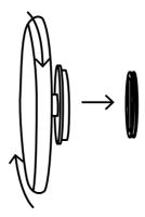
Wearing gloves so as not to mark the surface, position the Goldie Wall Plate over the bracket with the grub screws at the top and bottom.
