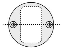
Using the Wall Bracket, mark out the location and level on the wall. Mark out the fixing points and central cavity by drawing around the inside of the rectangle.
