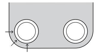
In an event when the legs should move after installation the leg should be 75mm inset from the table edge.
