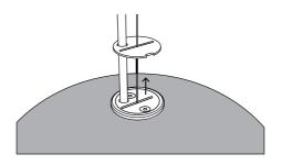
Ensure pendant is hanging level. The pendant can be adjusted laterally using the slot on top. Support the pendant while moving the steel cable along the ridged slot, allow slack in the cable to move into each compartment.
