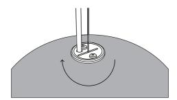
4 Rotate the outer shade around the suspension assembly to allow for levelling in all directions. Tighten screws back into top and replace cap.
