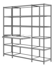
With at least three people, carefully lift the unit into an upright position. Once vertical place the remaining shelves into the unit, fixing in place with the bolts provided.
