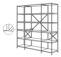
**4** Fix completed unit to a structural wall using the cross brackets and appropriate fixings.
