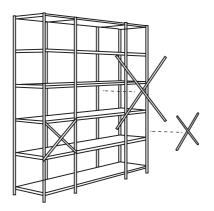
**3** To secure the unit fasten all cross brackets to the back of the unit using the bolts provided.
