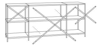
To secure the unit fasten all cross brackets to the back of the unit using the bolts provided.
