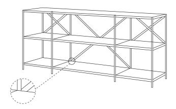
Fix completed unit to a structural wall using the cross brackets and appropriate fixings.
