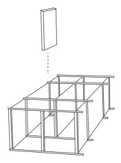
Place each of the frame uprights on a well padded surface with the screw holes facing down. Using an Allen key and the bolts provided fasten each of the shelves in place. Be careful not to over-tighten bolts if using an electric drill.
