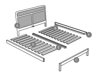
Unwrap and familiarise yourself with all the components. Both the headboard A and the foot rail C will have brackets pre-fixed to align and fasten the center rail. When arranging the frame please note the side rails B and center rail E are directional. Align so all the threaded inserts G are at the headboard end.
