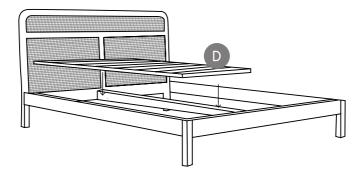
Unroll the slats D using the dowel attachments at each end of the frame as locators to hold the first and last slat in place. Repeat for the second slat roll.
