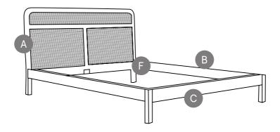
Headboard A and the foot rail C are now fastened together. If required tighten rail bolt fasteners F at each corner of the bed frame using the 5mm Alen key.
