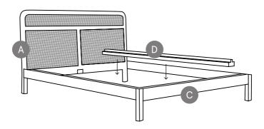
Place the center rail E by aligning the holes on the underside of the rail to the pins on the bracket attached to the bed frame at A and C.
