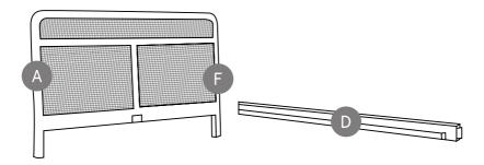
Push the headboard A and the foot rail C into the side rails B. Insert rail bolt fasteners F at each corner of the bed frame and tighten using the 5mm Alen key.
