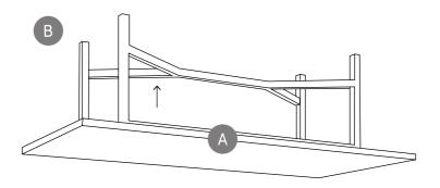
Place table top B carefully onto the base A. Ensure the top B is positioned correctly and in the middle of the base. Note: There is a X marked on top B and on the inside of the base A to assist you with placing the table the correct way.
