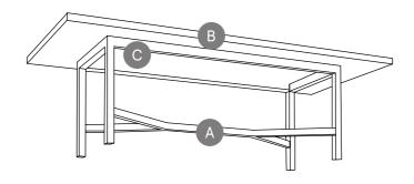
Fit the table top B onto the table base A by securing with the screws C. Repeat this process on all screw holes in the base A. Make sure the screws are tight to avoid bowing.
