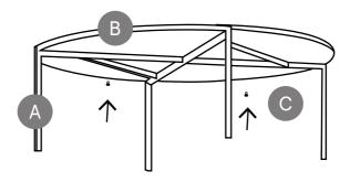
Using M6 Bolts C provided, screw through the base A into the top B to secure it.
