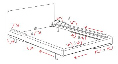
Screw timber feet D into metal plates located on the underside of each side rail B. Lay the loose cover G over side rails B and foot rail C. Align and straighten all seams on the corners. Remove velcro protecting strip from all around the inside of the cover (top part only).
