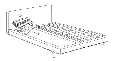
Fit center rail F to headboard A and to foot rail C using the allocated connection. Roll out slat rolls E, securing in place with the velcro attachments at each end.
