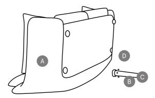
Line up the leg B and leg plate C to the sofa plate D. Using the 4 x M6 Bolts attach the leg plate C to sofa plate D. Ensure the leg straight edge is facing inwards. Note: Leg B and leg plate C will come assembled. Sofa plate D will be attached to the sofa frame A.
